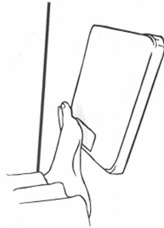
*Cover the solar cells for less than 1 second.*
